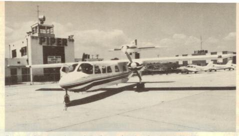
If, as some claim, two engines are better than one, how about three instead of two? The three-engine BN-2A Trislander is a growth version of the 10-place twin-engine Islander now used in over 50 countries. It incorporates more than 75% of the parts used in the Islander and is aimed at corporate aircraft operators and others who want considerable seating capacity, short-field capabilities, and comparatively low operating costs.
